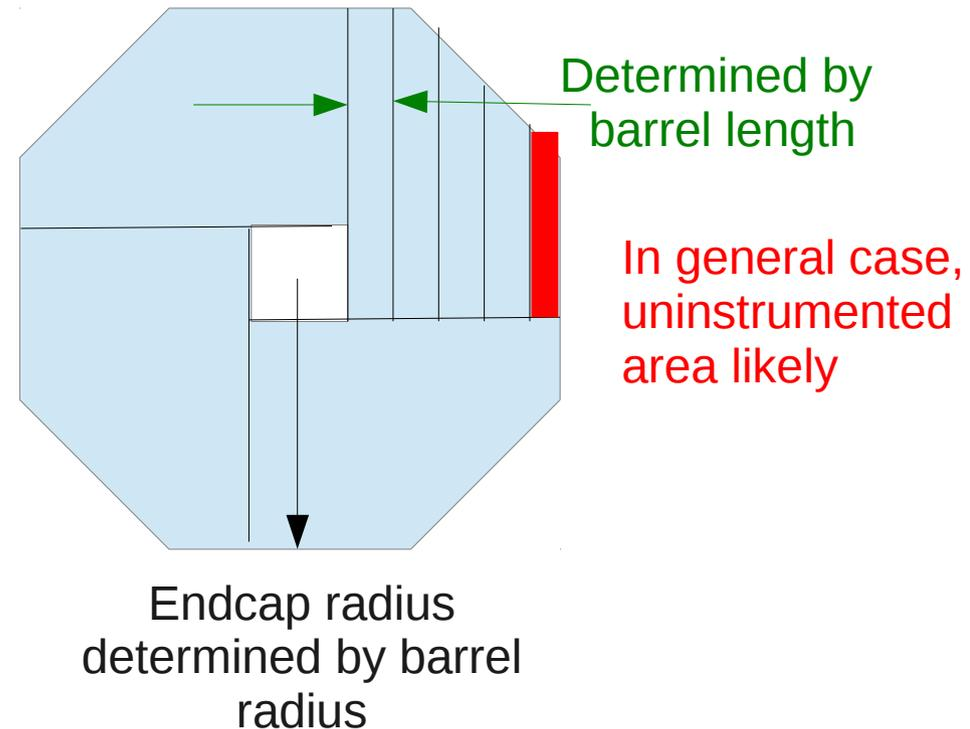
Can be large effects in scintillator, non-standard silicon ECAL geometries
