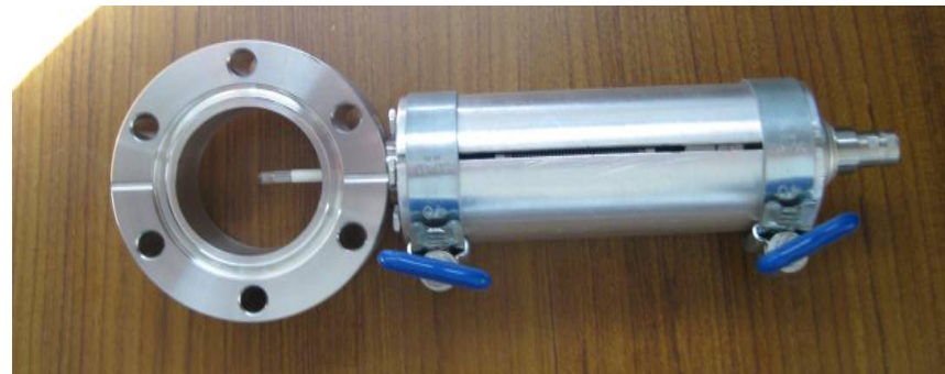
Aluminium tube and clamp to hold the bellow
