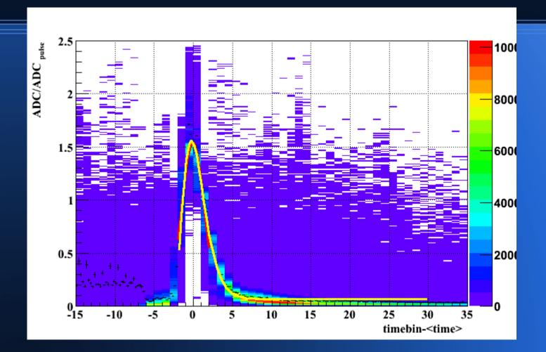
Defined in the same way as PRF Fitted with Gamma4 function (x^4exp(-4x)+noise)
