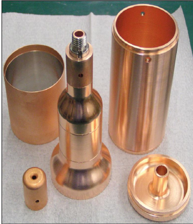
Inner conductor at cold side
