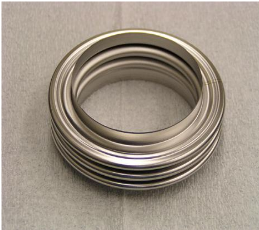
Bellows at cold side
