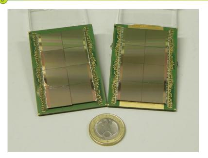
2 Oktoboards with bare Timepix chips produced and tested Modules is assembled GEMs tested (500 V @ N2 -> 0.7 nA leakage current) 380 V @ Ar:iButane 95:5 stands for ~30 min.
