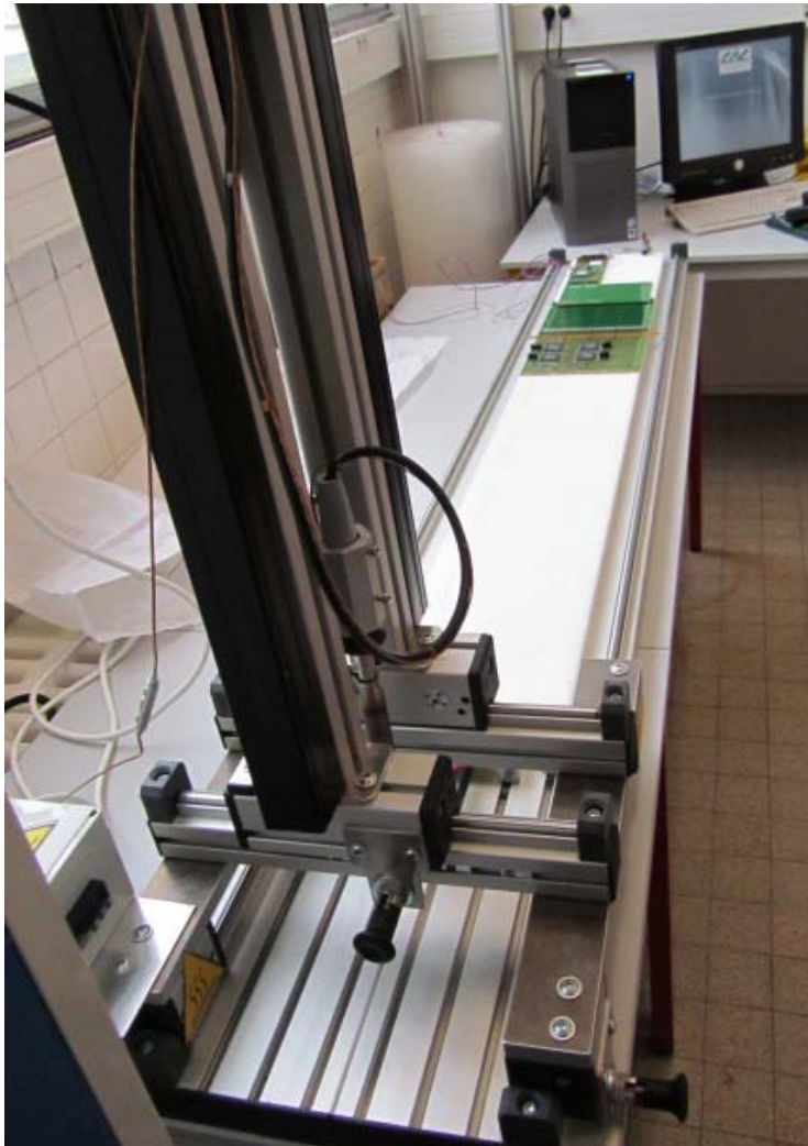
Solder bench with mechanical support length=1600 mm
