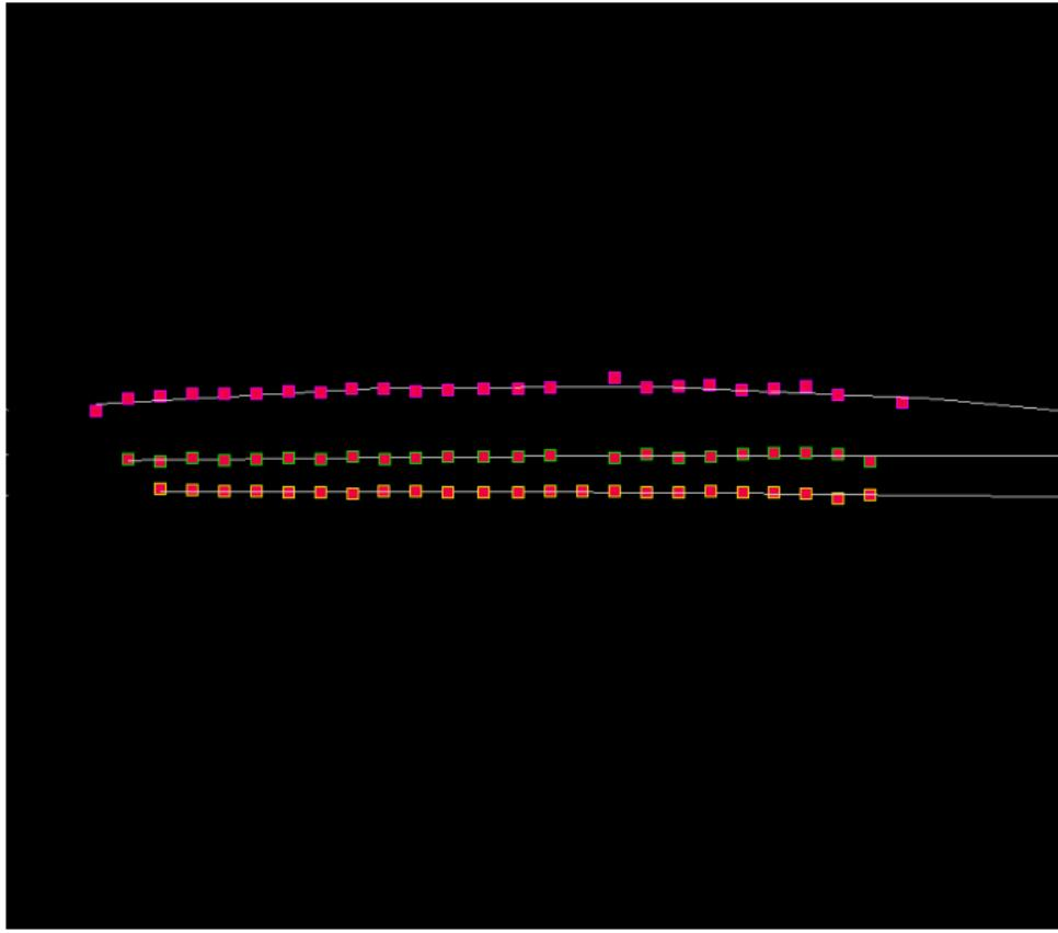
1-module data (June 2011), run 17637. 1 track has wrong direction (the IP is assumed to be far on the left ( $z = 0$ )):
