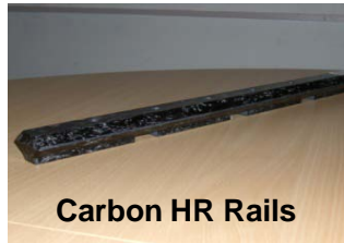
Opening in rails for cooling pipes and services on each column (EUDET) Ongoing development on sliding interface
