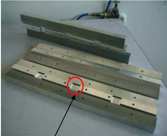
Opening in rails for cooling pipes and services on each column (EUDET) Ongoing development on sliding interface
