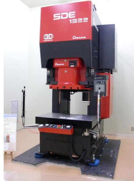
AMADA digital-survo-press SDE1522 150t, 50stroke/min, 225mmstroke
