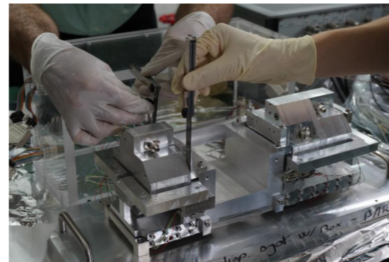
Mounting BPMs Adjustments w/ positioning tool (distance to IP plane, lateral alignment, yaw)
