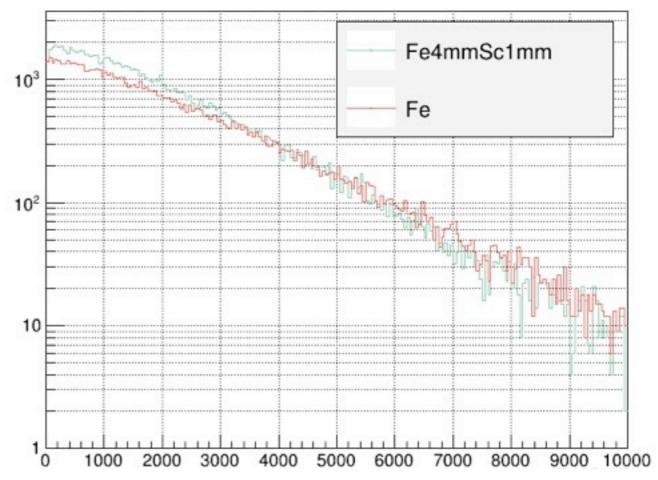
We see a 16.86% enhancement in the production of photons from neutron capture when adding plastic as active material.
