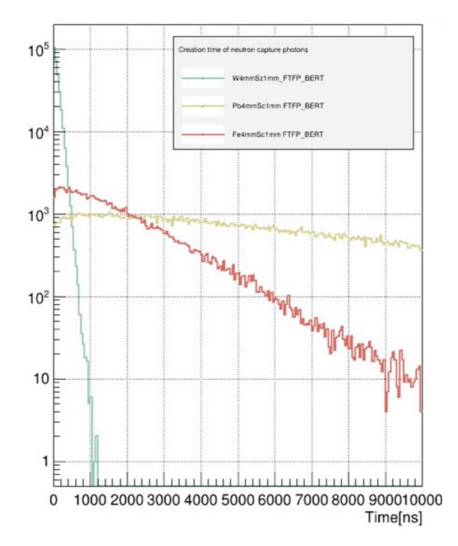
It takes longer for neutrons to thermalize in Pb as compared to Fe, and W (where this process is prompt).
