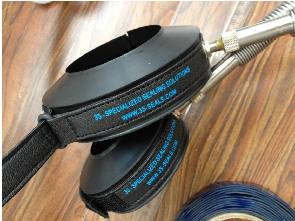
Figure 5: Rubber clamshell used for leak-check. The clamshell split is clearly visible in the larger, top, unit.
