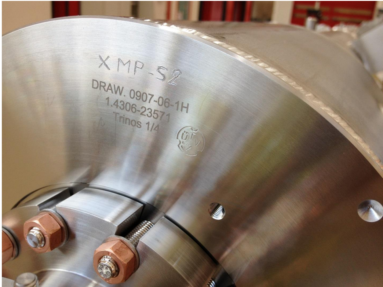
Figure 12: The end of the Ti tank, showing the weld, TÜV stamp and flange hardware.
