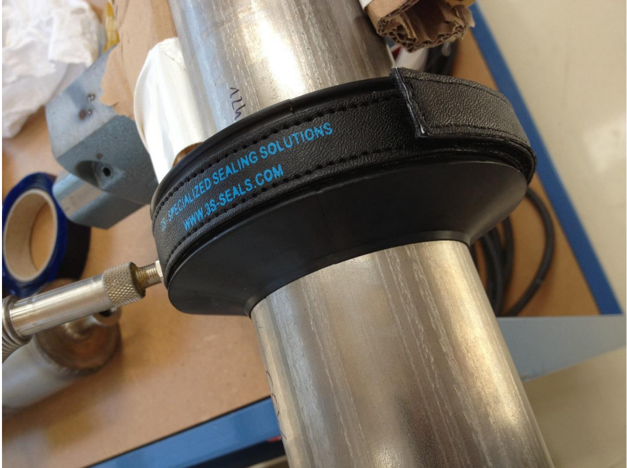
Figure 6: Clamshell leak-check device pumped down around a two-phase pipe weld.
