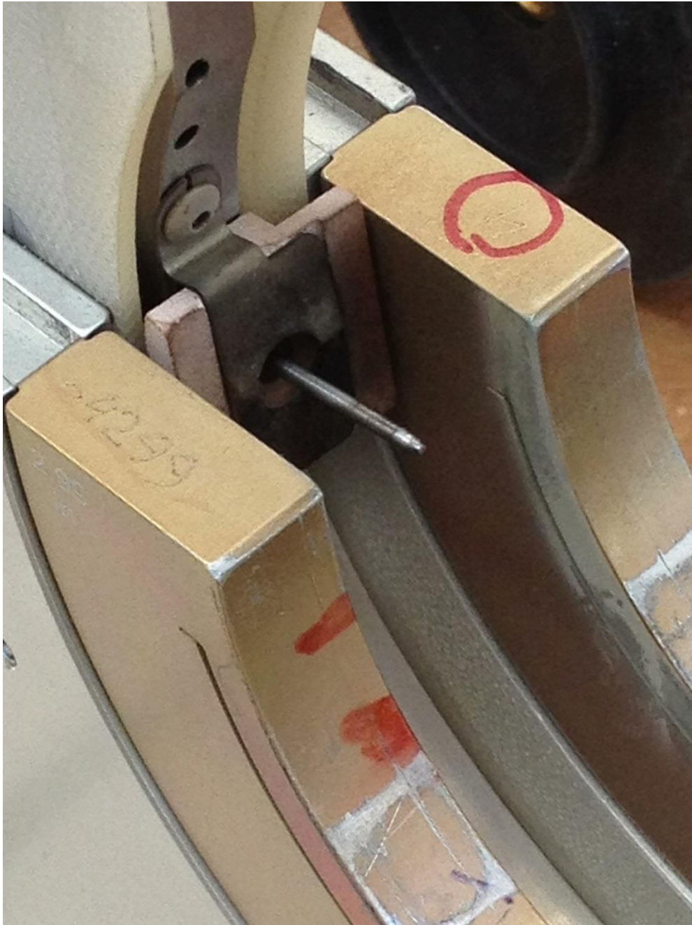
Figure 8: Tungsten electrode of the orbital welder. Two electrodes are required for a string. The electrode must be replaced by a qualified welder.
