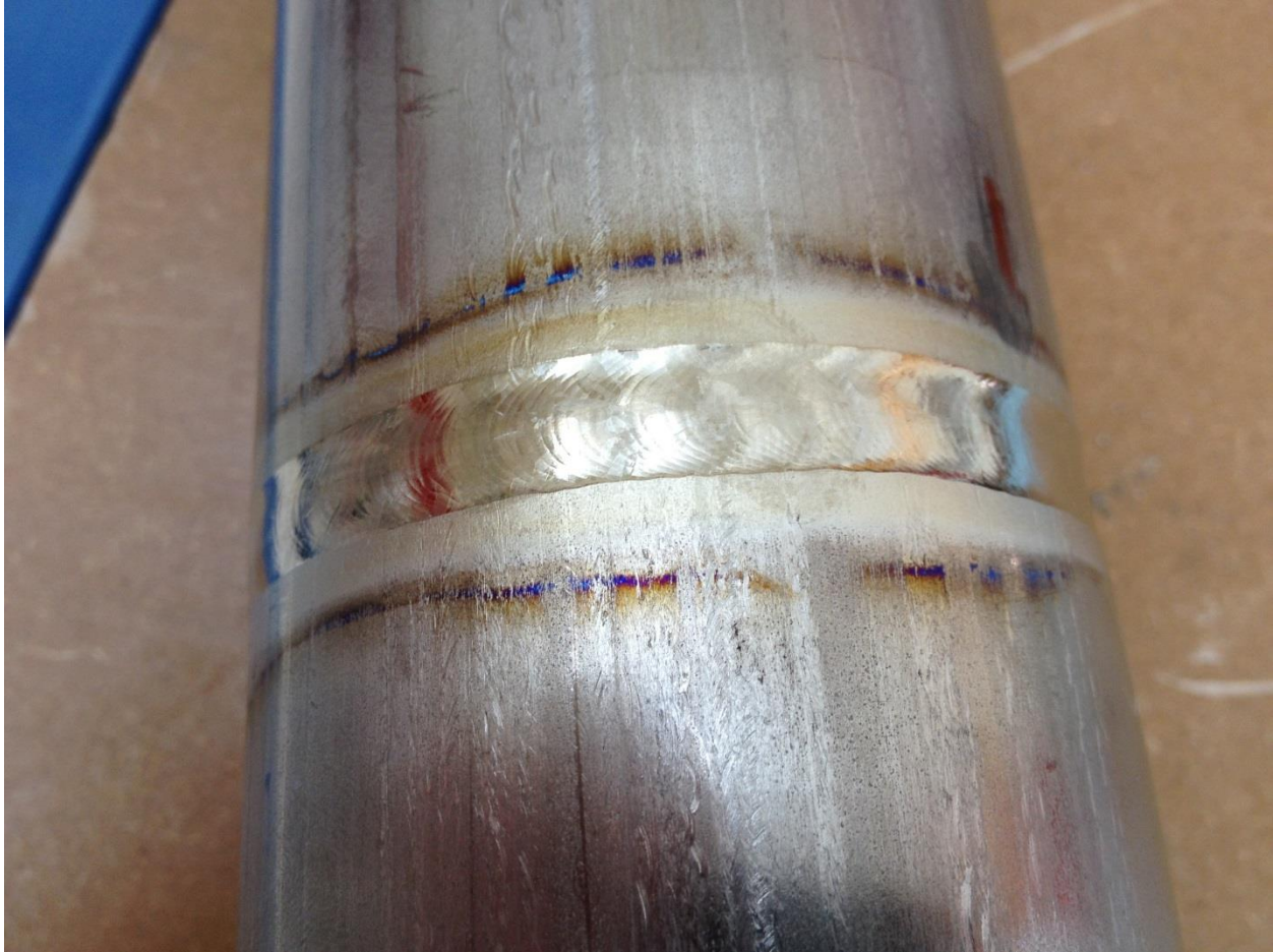
Figure 10: Ti two-phase pipe orbital weld results. The smooth ripples from the welder pulsing can be seen. Also light oxidation at the edge of the weld heat – affected zone can also be seen.
