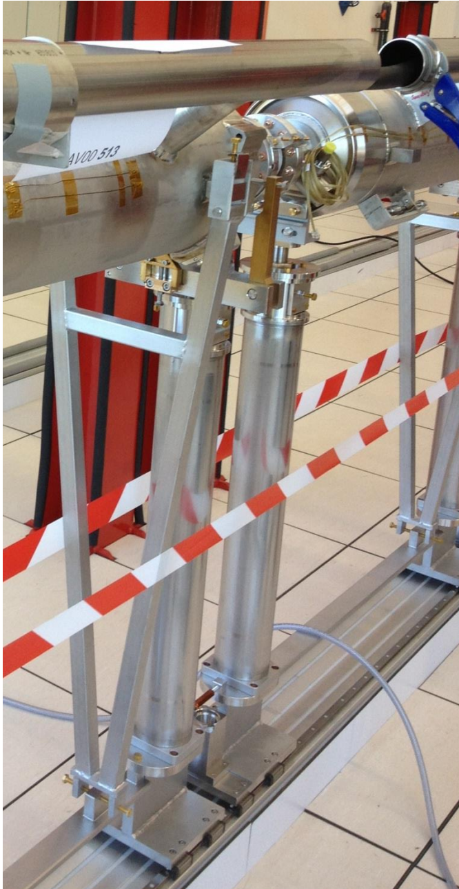
Figure 1: Inverted 'A' frame. This device and the quadrupole mounts are the only string roll-restraint.
