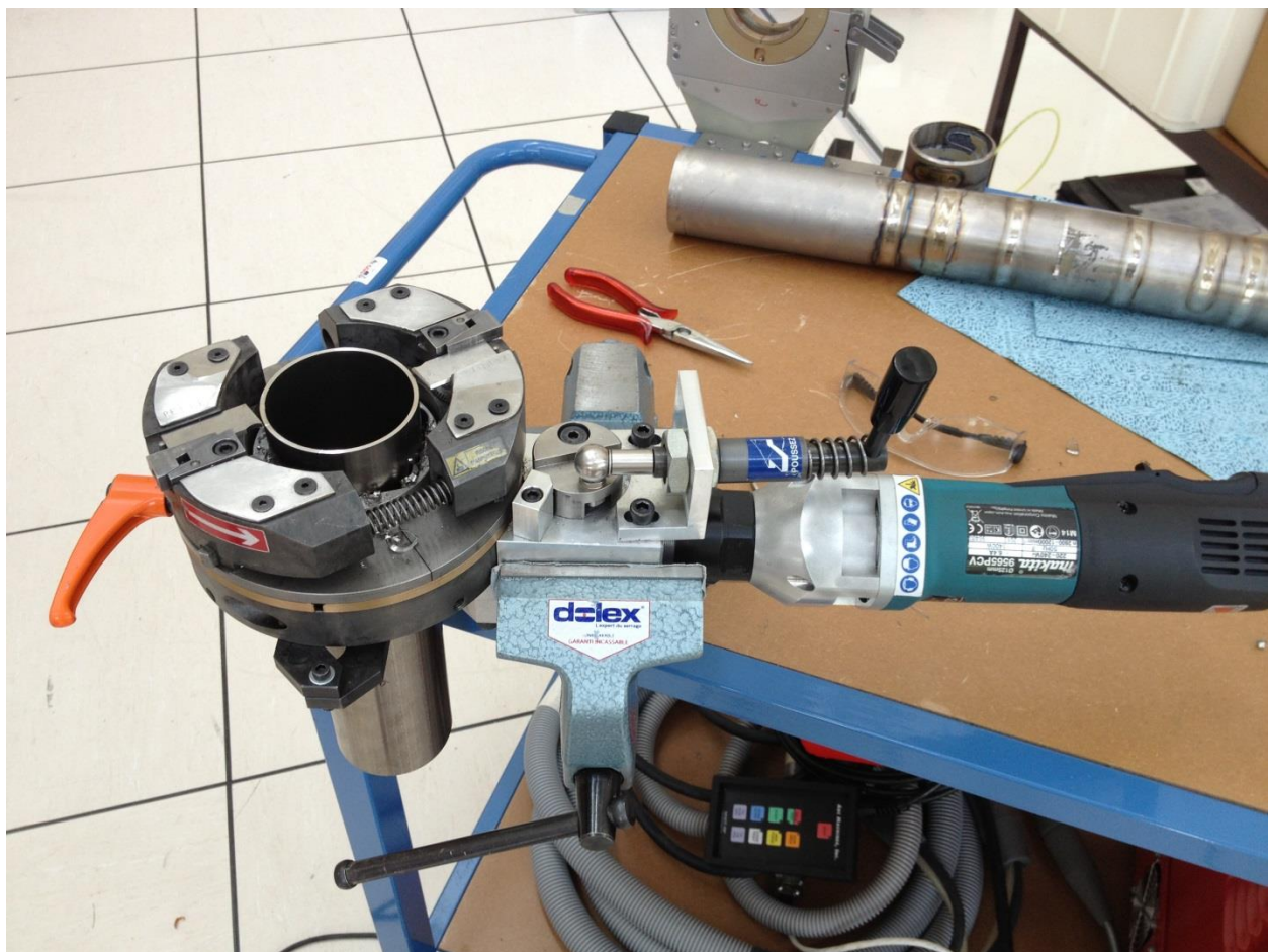
Figure 2: Electric automatic tubing trimming tool – test cut procedure. The drill-motor is visible on the right side. The large central handle in the middle of the
