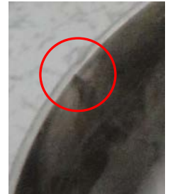
IHEP-02: quench defect has sharp and deep grain boundary step made during half cell pressing.
