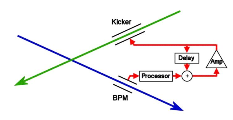
use strong beam-beam kick to keep beams colliding
