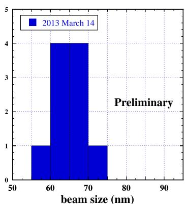
Beam size evaluated assuming no systematic error of the beam size monitor.
