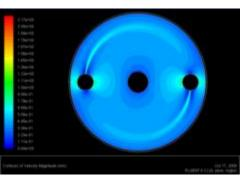
Velocity contours (inlet velocity: 2.17m/s, mass flux: 19kg/m/s) Maximum temperature variation as a function of time at  $z = 2.9m \equiv 8.1 \text{ X}_{\odot} \text{ Q}_{\odot} \text{ Maximum temperature} = 155^{\circ}\text{C}$
