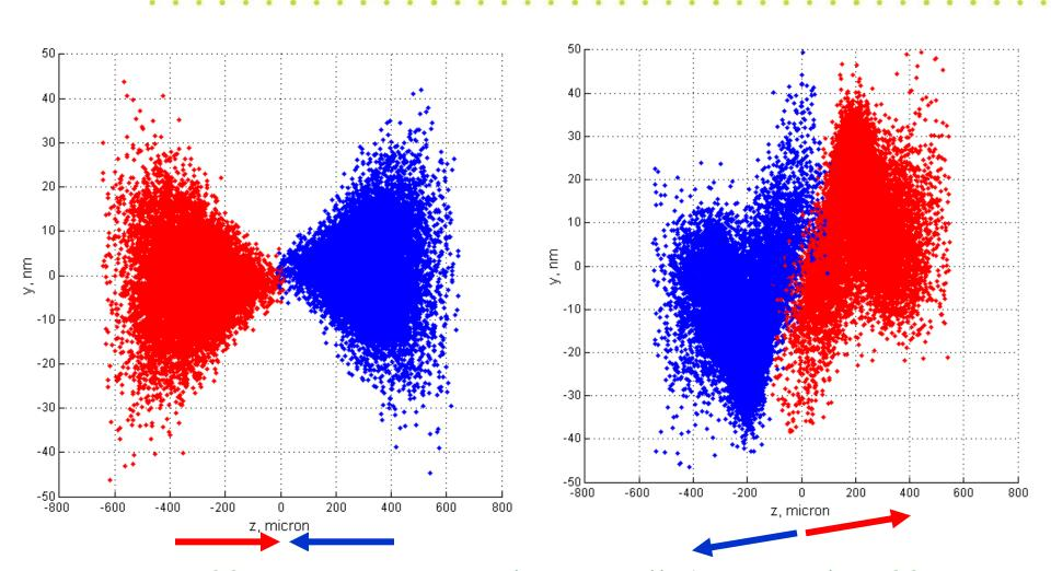
Sub nm offsets at IP cause large well detectable offsets (micron scale) of the beam a few meters downstream
