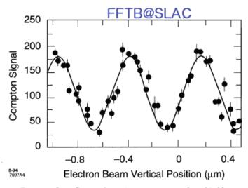
Figure 5.6: Laser-Compton beam size measurement performed in May of 1994. The measured size is 77±7 nanometers.
