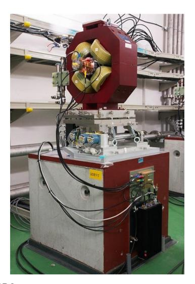
Cavity BPMs and SLAC front-end electronics modules provide submicron resolution of beam position
