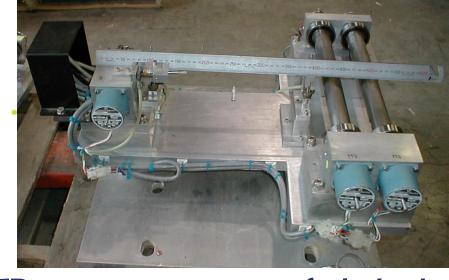
FFTB cam movers were refurbished and used for all and magnets of ATF2 (except bends)
