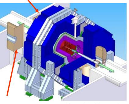
Detector and beamline shielding elements
