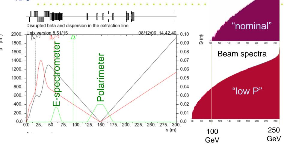
Extraction optics need to handle the beam with ~60% energy spread, and provides energy and polarization diagnostics
