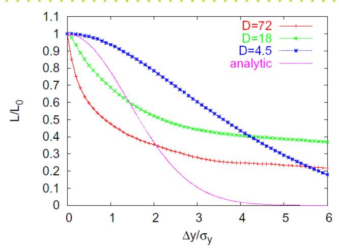
Luminosity (normalized) versus offset at IP for different disruption parameters
