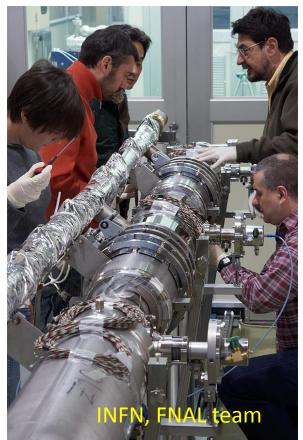
Tuner installation for FNAL, DESY cavities at outside of clean room
