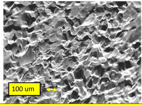
Simpler than EP, but the surface is rougher than EP. The roughness is coming from the difference of etching among the grain. Steps are made along the grain-boundary.
