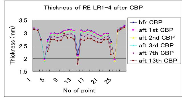
Thickness measurements by ultrasonic thickness gauge
