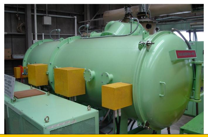
Annealing / degassing furnace at KEK: Two 9-cell cavity can be processed at once. Designed to consider about the supper-structure (Super-structure is consisting of two connected 9-cell cavities with one input-coupler).
