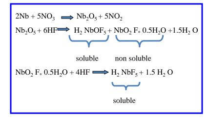
Exothermic reaction Removal rate ~ 2 µm/min @ 10C
