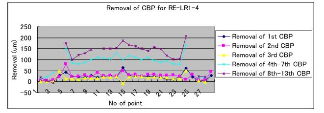
Removed weight 1<sup>st</sup> CBP: 21.0 g 2<sup>nd</sup> CBP: 21.0 g 3<sup>rd</sup> CBP: 16.5 g 4<sup>th</sup>-7<sup>th</sup> CBP: 78.0 g 8<sup>th</sup>-13<sup>th</sup> CBP: 94.3 g Total of removed weight = 230.8 g
