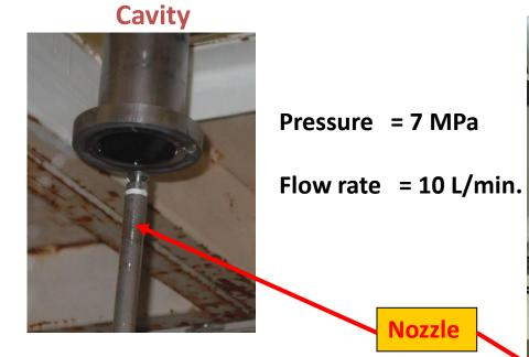
Ultra Pure Water Specific resistance = 18 M Ohm cm TOC = 10 – 20 ppb Bacteria = 0 – 3 count / mL
