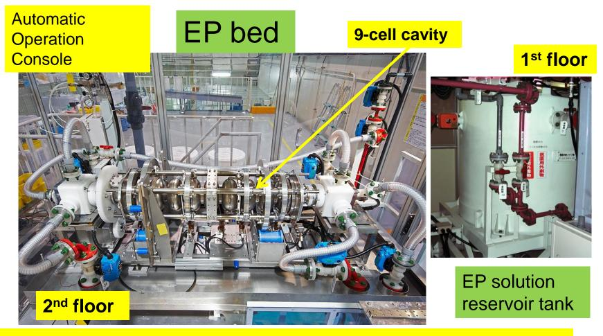
EP facility at KEK EP acid: HF + H<sub>2</sub>SO<sub>4</sub>, Aluminum anode, surface removal speed: 20µm/hour, V ~18V, I ~270A, T ~30degC (for 9-cell), cavity rotation: 1 rpm.
