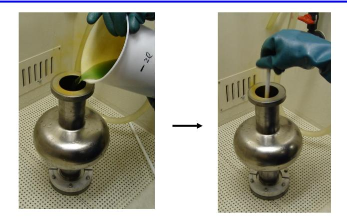
Components of BCP acid (KEK recipe) HF (HF 46%) :  $HNO_3$  (HNO<sub>3</sub> 60%) :  $H_3PO_4$  ( $H_3PO_4$  80%) = 1 : 1 : 1 (Volume Ratio)  $H_3PO_4$  can be increased if you like slow etching (1:1:2, 1:1:3, etc...)
