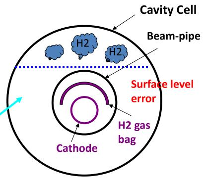
Failure of surface level of EP acid causes no accumulation of H2 gas.
