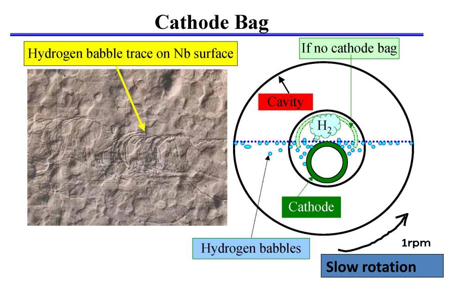
Hydrogen-gas bag should be set on the cathode appropriately. Otherwise, hydrogen-gas goes into the inner wall of cavity and causes Q-disease.
