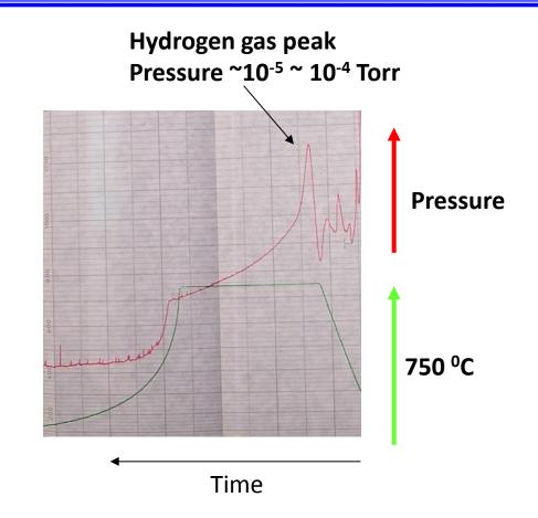
KEK recipe : 750 °C, 3 hours. Hydrogen gas can be degassed. Hydrogen in the Nb material cause Q-disease that degrade the Q value.
