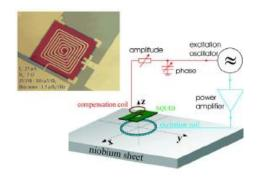
Low Tc superconducting SQUID system for eddy current testing of niobium sheets is in development
