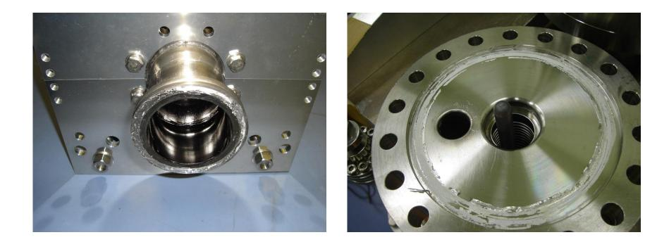
Indium is soft material. So the operation is complicated. Even when disassembly of cavity, the removal of indium is not easy work. And because the melting point of indium is low : T = 156 C, you should pay attention to the temperature control of In-situ baking (T=120 – 140).
