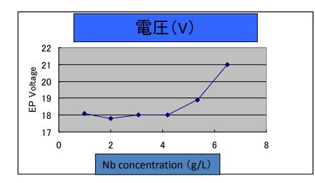
Repeating EP processes under the constant current density( = 50mA/cm<sup>2</sup>).
