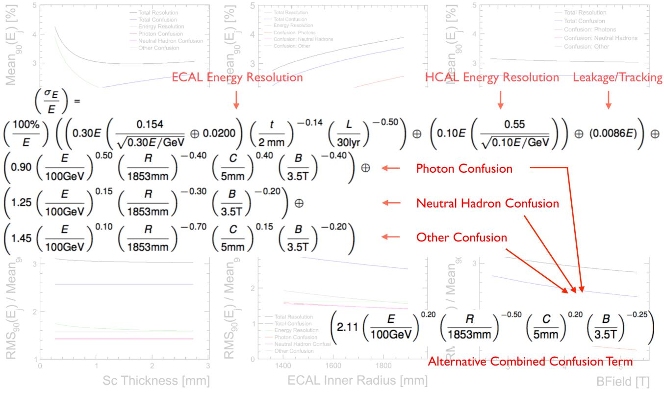
Parameterisation can be used for a ScW or SiW ECAL. To use with SiW ECAL, remove references to cell thickness variation and alter basic ECAL energy resolution.
