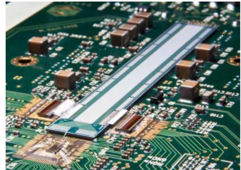
Long drain lines  $\sim 60$  pF parasitic capacitance
