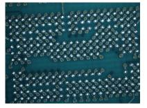
Figure 2: A Carrier Board with bonded SALTRO-chip (top-left) and a blow up of one corner (leftbottom), where the bonding wires can be seen. To the right the bottom side is shown whith small tin balls applied.
