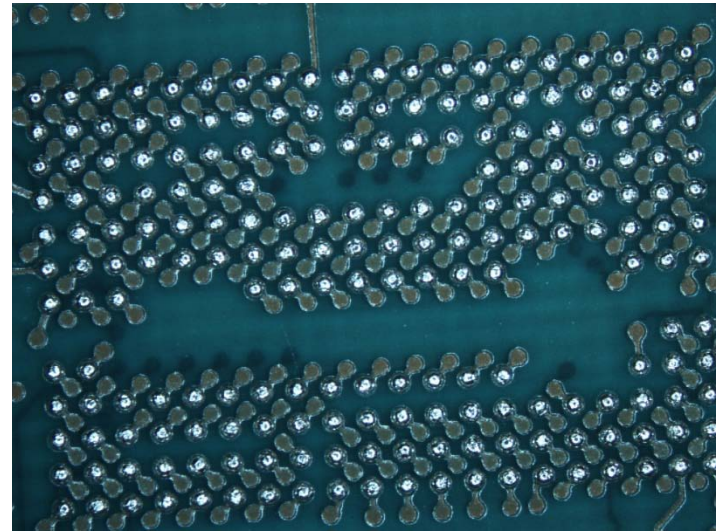
Bottom side of the Carrier Board with tin balls
