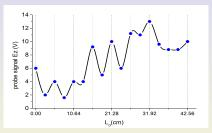
Probe signal at the end of vacuum part of dielectric unit[V.A.Kiseljov et al]
