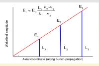
Process of wakefield setting. Axial distribution of wakefield amplitude in matched DWG: at left - initial state when 1st bunch has reached the WG end, at right - stable state
