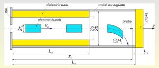
Geometry of DWG. Choke and tube are fabricated from the same material.
