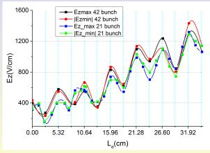
Max and min of  $E_z$  at  $z = 0.9L_s$ , r = 0 versus  $L_d$  for different number of bunches in the train. Vertical grid lines are drawn every  $\lambda/4$
