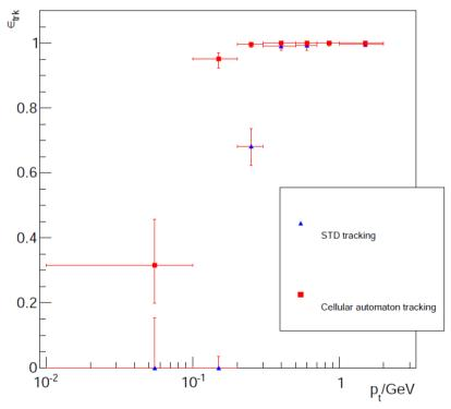
Efficiency for higgsino sample + pair bkg for a proposed CMOS VXD, std vs new tracking algo
