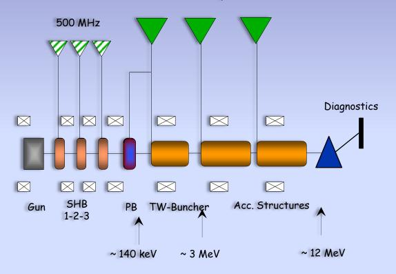
Major components under development, gun, SHB, PB, TW-Buncher As well as power sources, up to 100 kW, wide band solid state source at 500 MHz and 20 MW L-band klystron with 70 % efficiency (two prototypes have been ordered with Thales and Toshiba)
