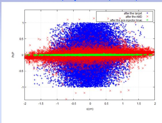
Phase space after target, after AMD and at the end of the 200 MeV pre-injector linac using CDR parameters
