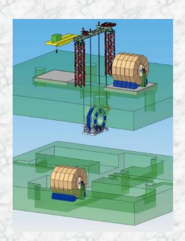
Vertical Access (in addition to horizontal) (CMS-like. Kitakami site allows this)
