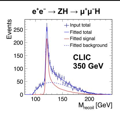
HZ events can be identified from Z recoil mass  $\rightarrow$  model independent measurements of the g<sub>HZZ</sub> coupling
