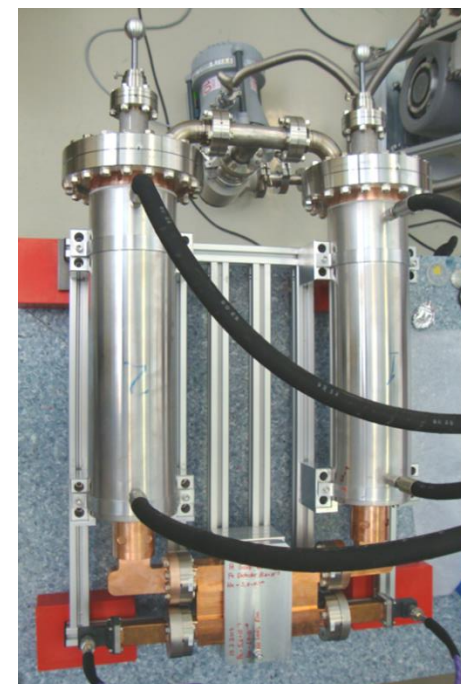
SLEDX RF pulse compressor. Built at CERN.
