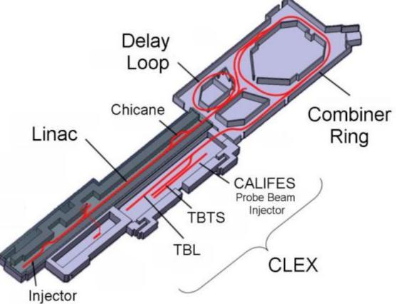
From injector to two-beam experiments and CLIC prototypes test line to general instrumentation test line. Already happening?
