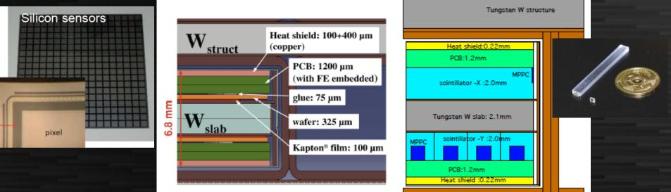
Tungsten absorber + Silicon Tungsten + Scintillator strips 320 μm (maybe 500 μm) 5 x 5 mm<sup>2</sup> pixels 256 pixels / chip Expensive sensor
