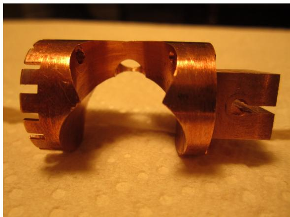
*After the insertion pieces will be inserted to OTR chambers, we expected to the wake field of OTR chamber will be symmetric for vertical direction.*
