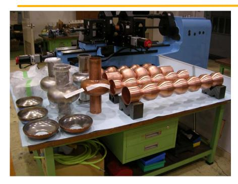
A 3 mm Cu/1 mm Nb bonded pipe undergoes necking and hydro-forming.
