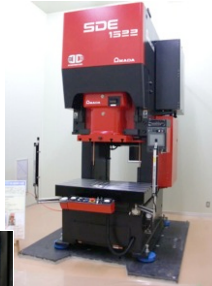
AMADA digital-survo-press SDE1522 150t, 50stroke/min, 225mmstroke
