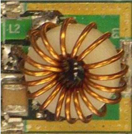
Toroid Inductor with Shield on toroid
