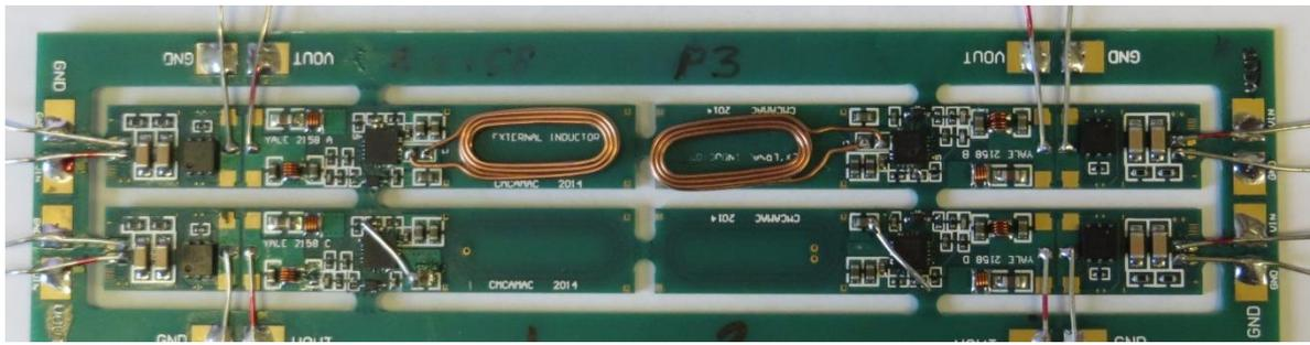
Each Converter PCB 10 mm x 63 mm. Different Coil Configuration
