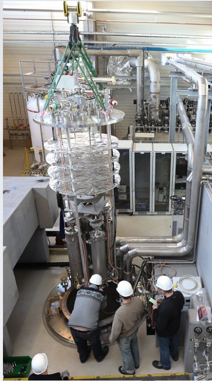
Vertical (accept.) Test (VT) at DESY AMTF
