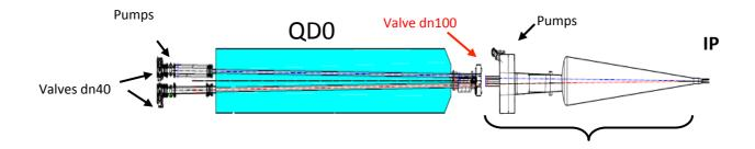
Need a pumping system between the two DN 100 valves (hot part of the IP chamber)
