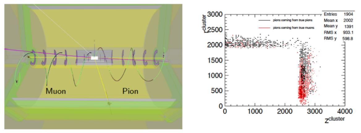
The particles curl and travel along the magnetic field lines, and hit the endcap calorimeters
