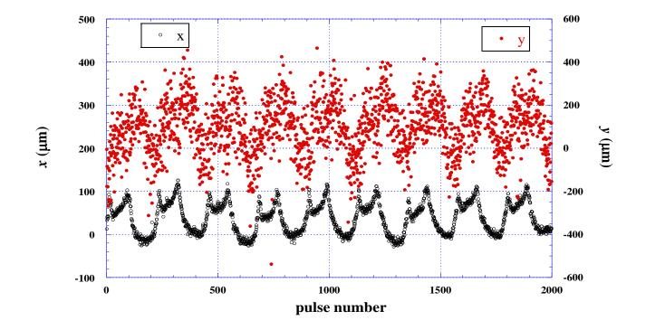
In horizontal, drift is larger compare with pulse to pulse jitter. In vertical, pulse to pulse jitter is more significant. (It may be only in this particular case. (?))
