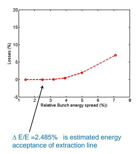
No Beam losses for initial rms relative energy spread equal to 1.75 times of nominal spread. (  $1.75 \times \sigma_E = 2.485 \%$ ).  $\sigma_E = 1.42\%$
