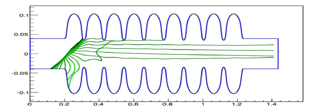
Emitter location: 7 mm us from the 1st iris, RF phases from 0 to 360° with the step of 5°  $\,$
