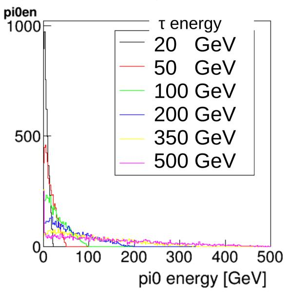
τ produced in Higgs decays near the e+e- -> ZH threshold are strongest motivation for reconstruction of τ decay modes ---> τ energy ~ 60 GeV,  $\pi^0$  energy typically few 10s of GeV
