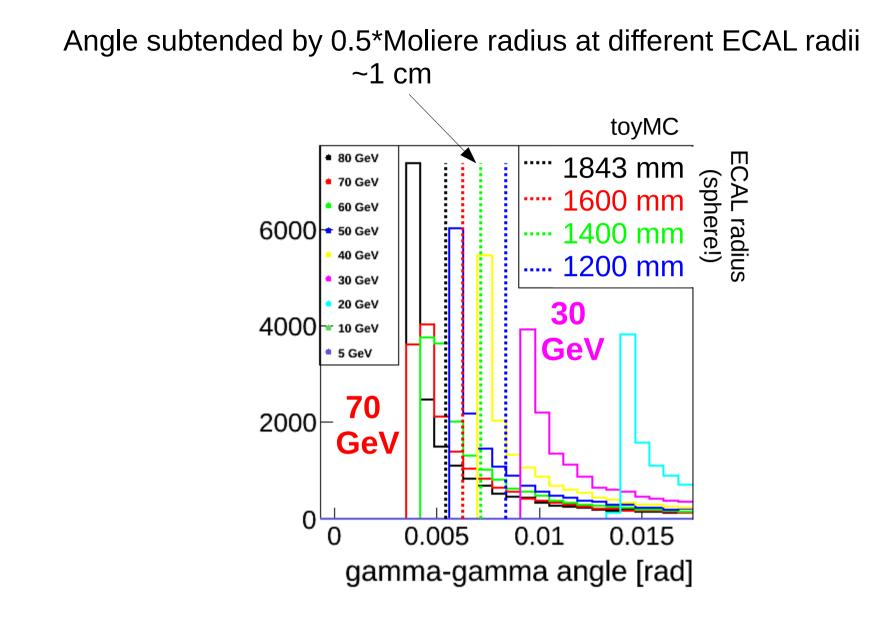
$\pi^{o}$  of 30 GeV and below should be identifiable in a typical ILC ECAL with a good photon separation algorithm  $\pi^{o}$  of 80 GeV look difficult
