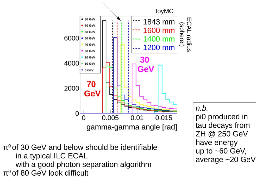
Angle subtended by 0.5\*Moliere radius at different ECAL radii ~1 cm
