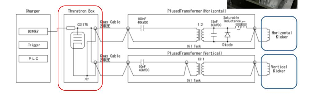
The power is always stored in the capacitors, we can generate the single kicker pulse, when the thyratron will be fired.
