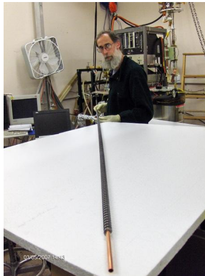
Undulator yoke under test at Cornell
