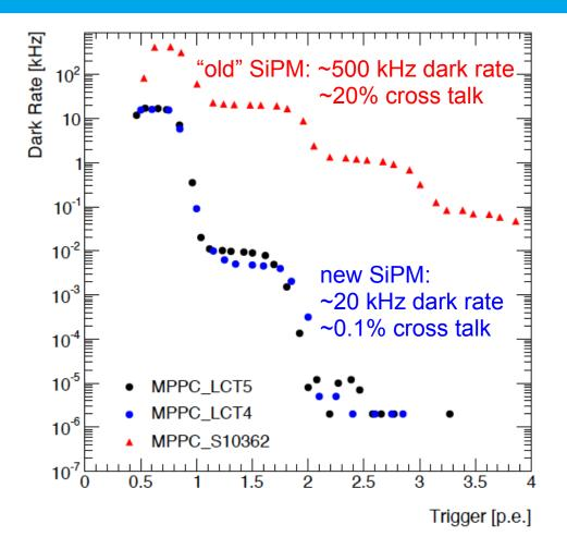
for comparison: SiPMs in physics prototype 2 MHz dark rate, 30% cross talk
