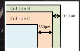
Cut sizes affect the breakdown voltage and leakage current
