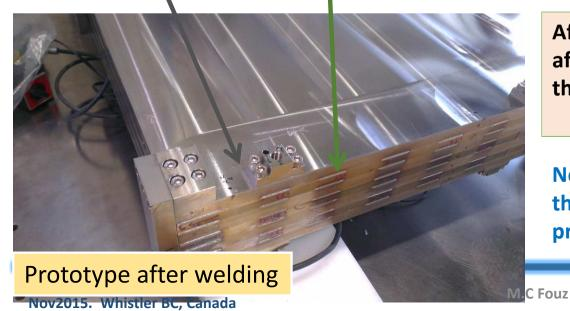
After comparing the measurements before and after welding deformations found (~1mm) bigger than expected in X-axis. O.K in Y-axis
