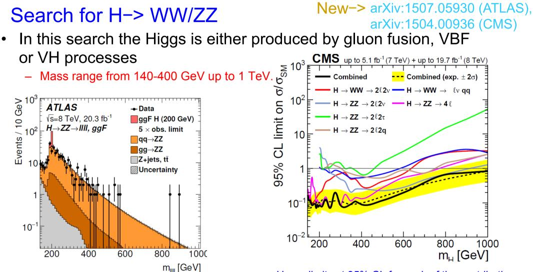
Distribution used in a likelihood fit of the fourlepton invariant mass ( $m_{IIII}$ ) for H->ZZ->IIII search in the gluon-fusion production mode. No events are observed beyond the upper limit of the plot. Upper limits at 95% CL for each of the contributing final states and their combination. The theoretical cross section,  $\sigma_{\rm SM}$ , is computed in arXiv:1307.1347.
