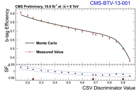
(Left) Inverse background efficiency versus signal efficiency for the offline tau identification.(Right) b-tagging efficiency as a function of the discriminator for the CSV algorithm.
