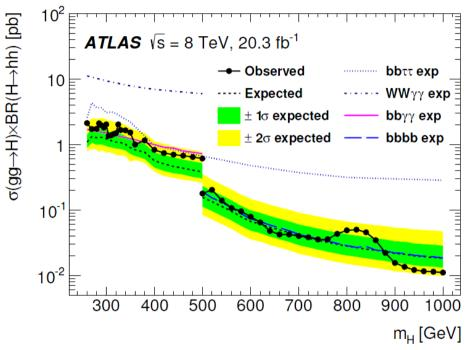
Results combining all channels. The improvement above 500 GeV is due to the sensitivity of the hh->bbbb channel.
