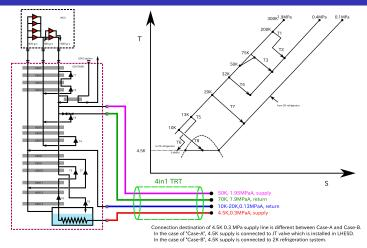
• In the case of "A", total shield length is very long (8km).  $\Rightarrow \Delta p$  in shield line should be less than 1bar to obtain correct inlet pressure of T3.
