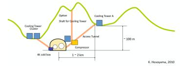
Only cooling towers on surface for effective heat removal, and others underground
