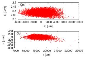
Final Emittances (2.5 turns):  $\gamma \epsilon_{x} = 111 \ \mu \text{m}, \ \gamma \epsilon_{y} = 107 \ \mu \text{m}$
