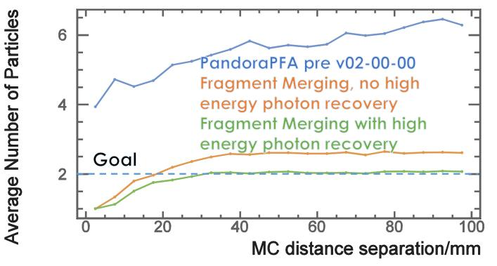
Average number of reconstructed particle as a function of distance separation, in barrel and end cap only
