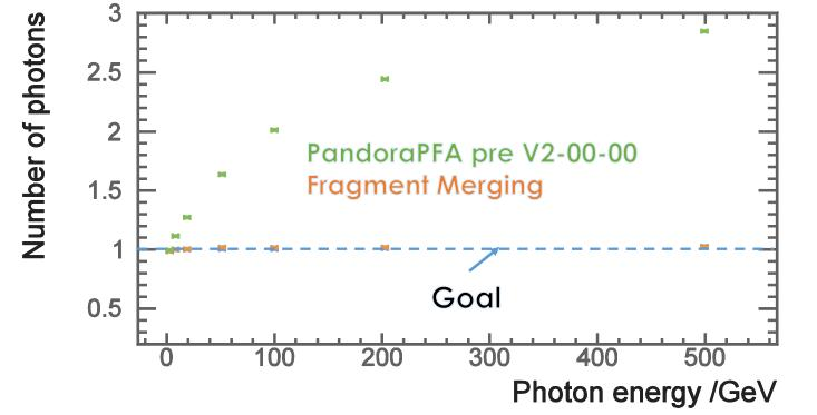
Average number of reconstructed photon as a function of photon energy at generator level
