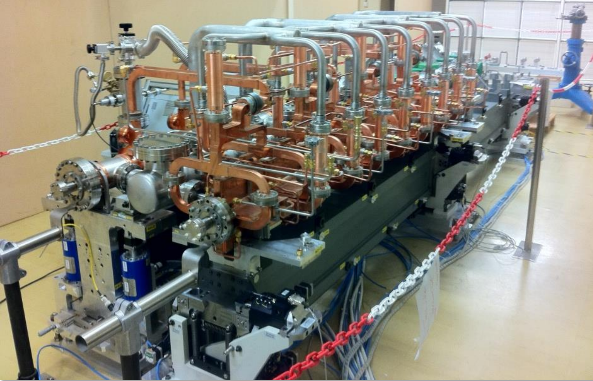
Module mechanical characterisation test stand: active alignment, fiducialisation + stabilisation (PACMAN)
