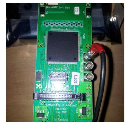
VMM1 chip : peaking time from 25 ns to 200 ns gain from 1fC/mV to 16 fC/mV : on going tests (nice pulses on the scope, need to check the DAQ now)
