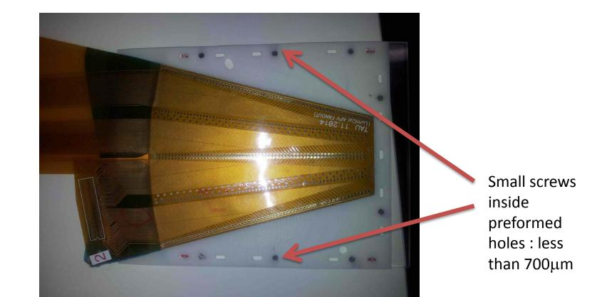
700μm sensor, HV and readout Panasonic connectors on kapton fanout
