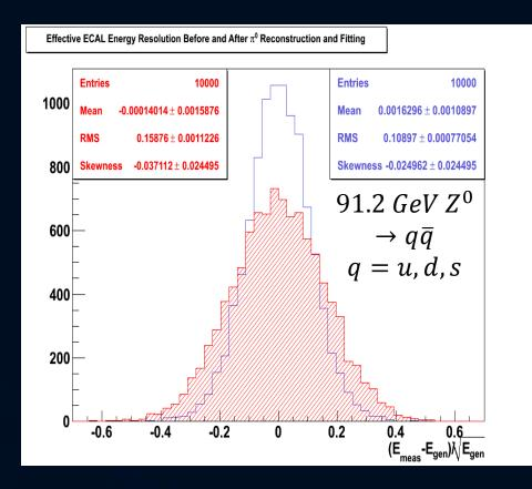
Photons account for on average 24.8 GeV of the total 91.2 GeV in the events
