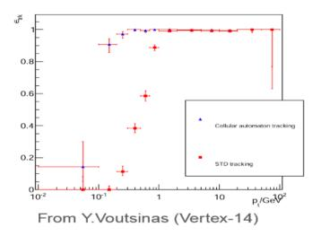
TPC has distinct advantage at low momenta because of lower material compared to Silicon tracking.
