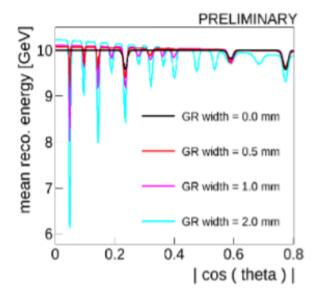
Reconstructed energy from ECAL vs. cos(theta): dips are from dead areas and guard rings in the Si sensors
